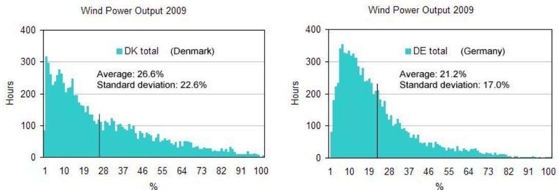
The average in Germany reflects the lower average wind intensity at the wind power sites. The standard deviation depends on the size of the country. It is obvious from the chart that Germany has a lower number of hours with very low and very high total output.
