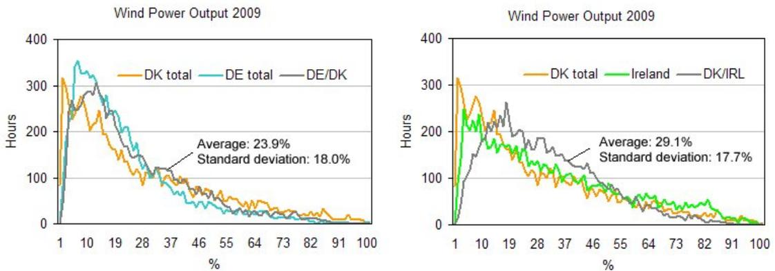
The left hand chart shows that only modest improvements have been obtained in a combination of Denmark and Germany. By combining Denmark and Ireland a different distribution function appears. The numbers of hours with output lower than 10% and higher than 60% have been counted. The upper and lower limits are arbitrarily chosen.
