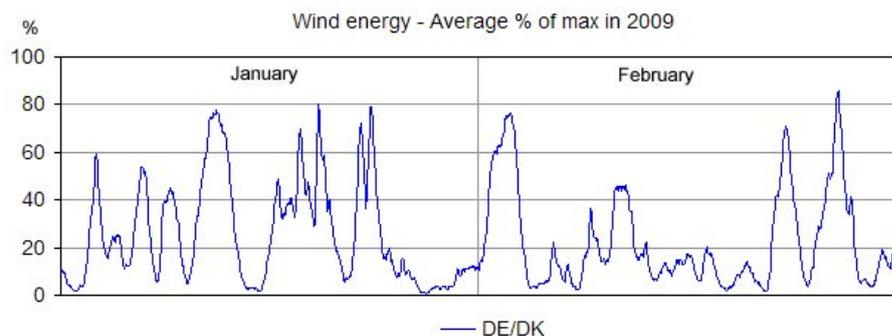
The chart shows the volatile and random nature, even for the average wind power output for Germany and Denmark. The duration of typical wind power waves can be between 2 and 4 days. The peaks are slightly lower than for each country, but there are still periods with very low generation and several days with less than 20 % energy output.
