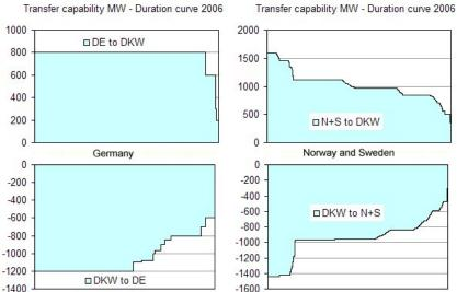
The HVDC links to Norway and Sweden suffered from severe hardware faults during 2006. There were capacity reductions most of the time. At the worst only about  $\frac{1}{3}$  of the nominal capacity was available.
