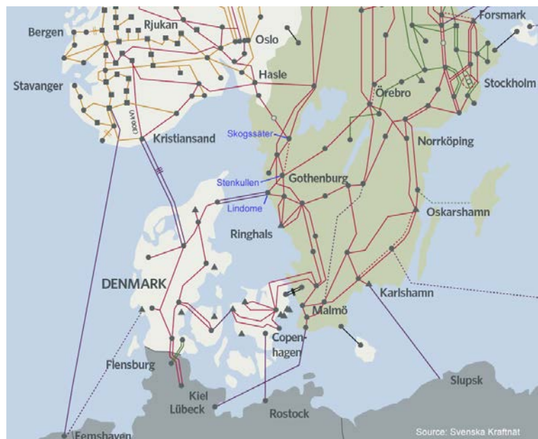
Fig. 8 - Reinforcements of the west coast corridor: Lindome-Stenkullen-Skogssäter
