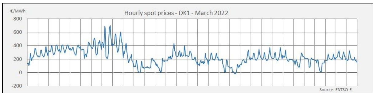
Fig. 7 - The spot prices (DK1) reflect the variations of wind power
