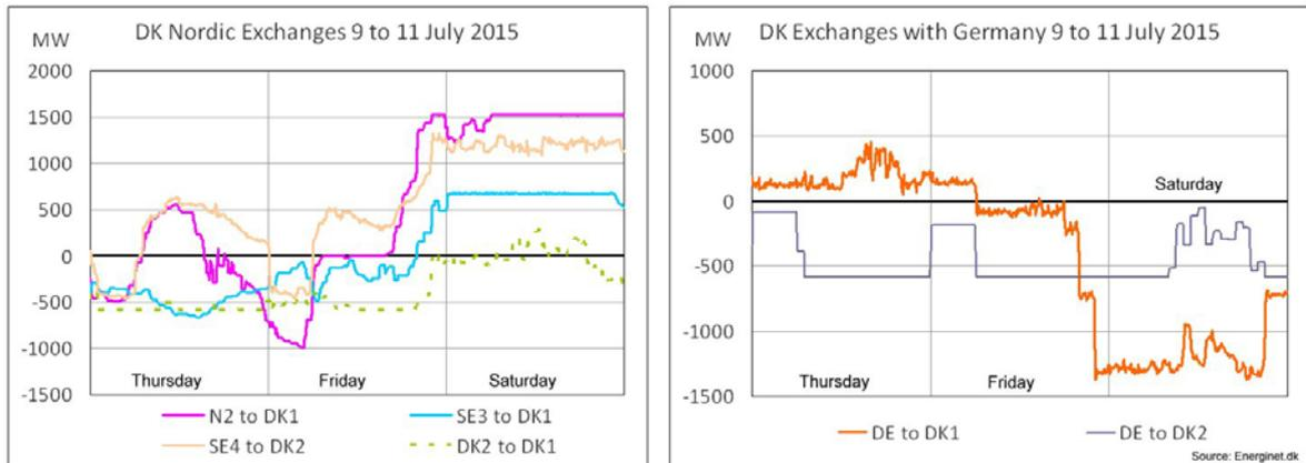
The left chart shows that exchanges with Norway and Sweden followed the wind power variations while the thermal units in Denmark were running at minimum production. During the Saturday there was a rather steady import at about 3,400 MW from Norway and Sweden while Danish thermal units balanced Danish load variations.
