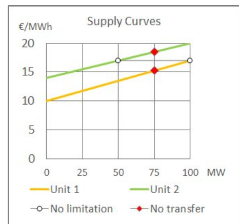
Fig. 4 - Two units with increasing supply curves
