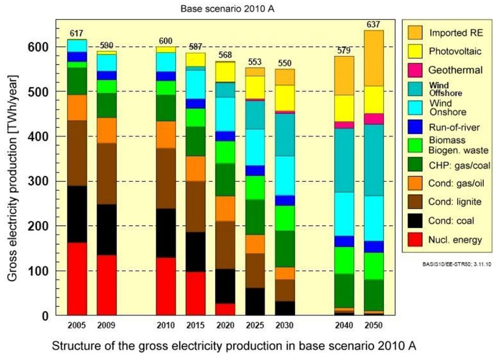
It appears from this graph that Germany is expected to import an increasing part of the electricity consumption. Even 80 GW of controllable capacity and 160 GW of variable capacity will be insufficient for covering the full demand in 2050.
