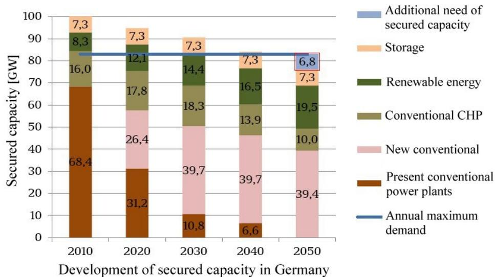
New conventional capacity provides 39.4 GW and CHP 10 GW. The 6.8 GW at the top is additional need for secured capacity.
