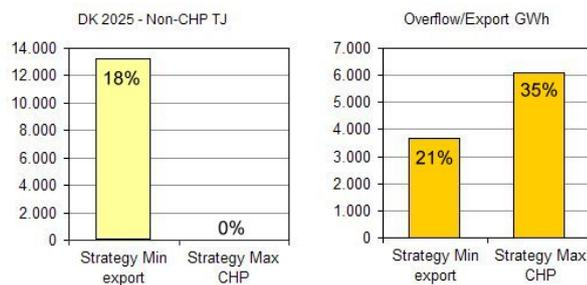
The result of the minimum export strategy will be export of **21%** of the wind energy and **18%** of the heat demand unsupplied by CHP. By maximizing the use of CHP **35%** of the wind energy output must be exported. *This is the starting point* for the subsequent experiments with different integration measures.
