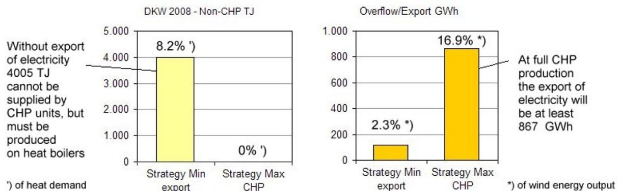
By *minimizing electricity export* only 119 GWh (**2.3%** of wind energy output) must be exported, but 4,005 TJ (**8.2%** of heat demand) cannot be supplied by the CHP units.
