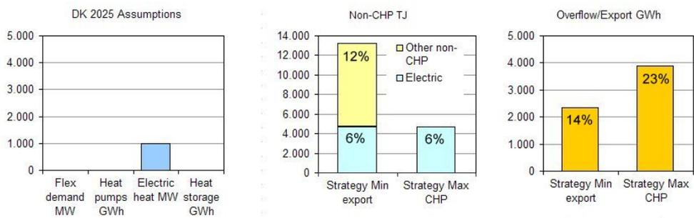
1,302 GWh (= 4,686 TJ) have been used for electric heating. It is an important condition for the validity of the result that all electric water heating can be justified by current market prices.
