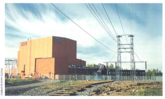
Full-scale line span erected at the Swedish Transmission Research Institute (STRI) at Ludvika. Test results show that it is possible to develop new methods for separating and suspending wires in power lines that will make the magnetic field approx. 90% weaker
